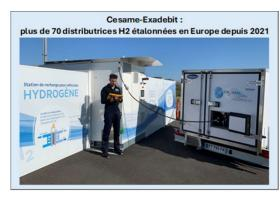
Building on this commitment, the company has, in recent years, developed mobile reference measurement systems for the calibration of hydrogen dispensers used to refuel vehicles. These systems comply with the OIML R139 recommendation and French regulations. Cesame-Exadebit is currently the only company in Europe accredited to ISO 17025 for this activity.
